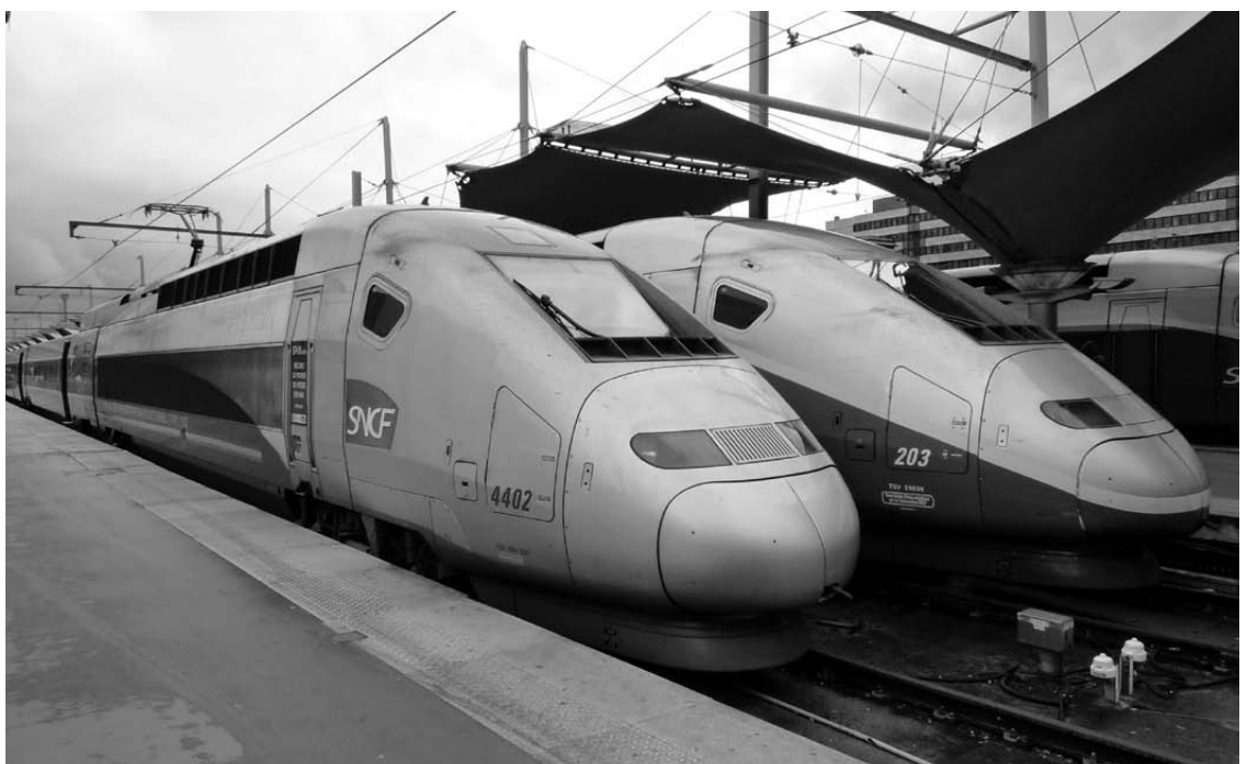
French TGV-POS and TGV-Duplex with top commercial operating speed of 320 km/h (world's fastest)
