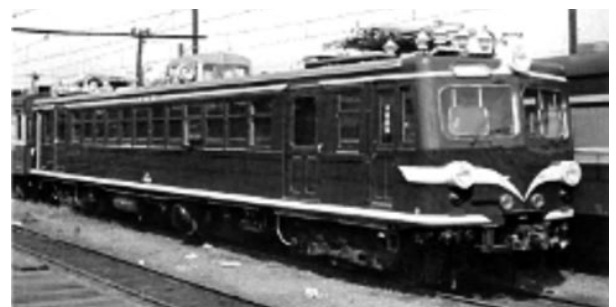
Kumoya 93 High-speed Testing Car that Set a Record of 175 km/h (100 Years of JNR Rolling Stock)
