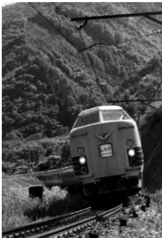
Series 381 Shinano limited express. This series was the first tilting EMU (A Hundred Years of Progress in JNR Rolling Stock)
