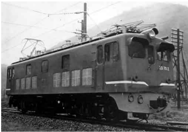
First mass-produced Class ED70 AC locomotive in 1957 (A Hundred Years of Progress in JNR Rolling Stock)
