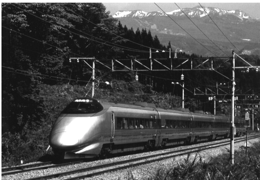
Series 400 for Yamagata-bound Tsubasa service with shorter body and smaller loading gauge (JR East)
