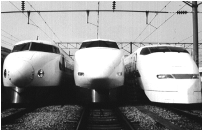
Series 0, 100, 300 standing side by side at JR Central depot. Series 100 has two or four intermediate double-deckers (S. Kubo)
