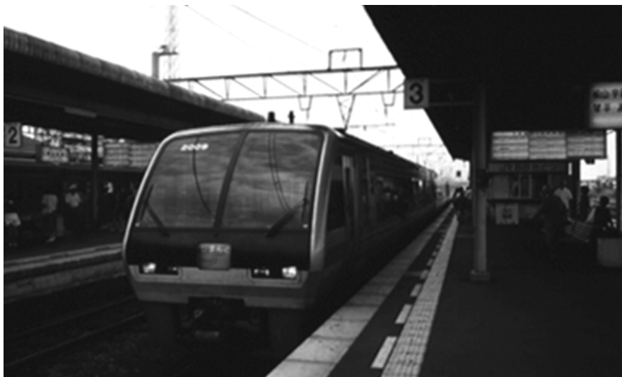
Series 2000 tilting DMU introduced in 1989 for rural limited express services
