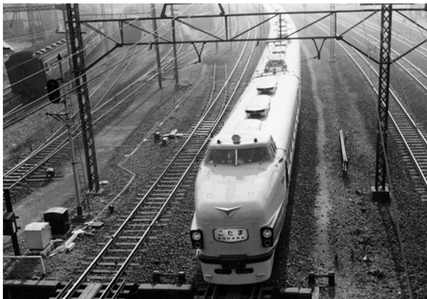
Moha 151-series express EMU used on the electrified Tokaido Line
