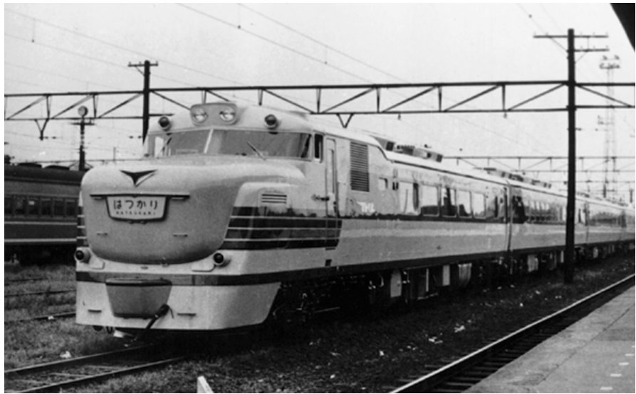
Kihō 81-series express DMU used on Joban and Tohoku Lines
