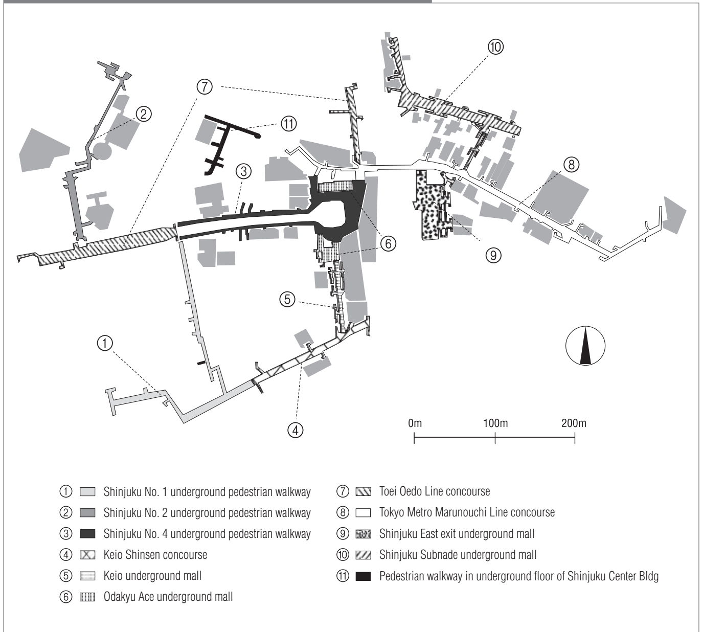
Figure 1 Administrative Sections of Underground Spaces at Shinjuku Station
