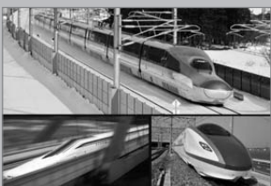
Shinkansen cars of Hokkaido, Chuo (using SCMAGLEV), and Hokuriku Shinkansen. Top: Series H7 car (Kotsu Shimbunsha), bottom left: Series L0 car (JR Central) bottom right: Series W7 car (JR West)
