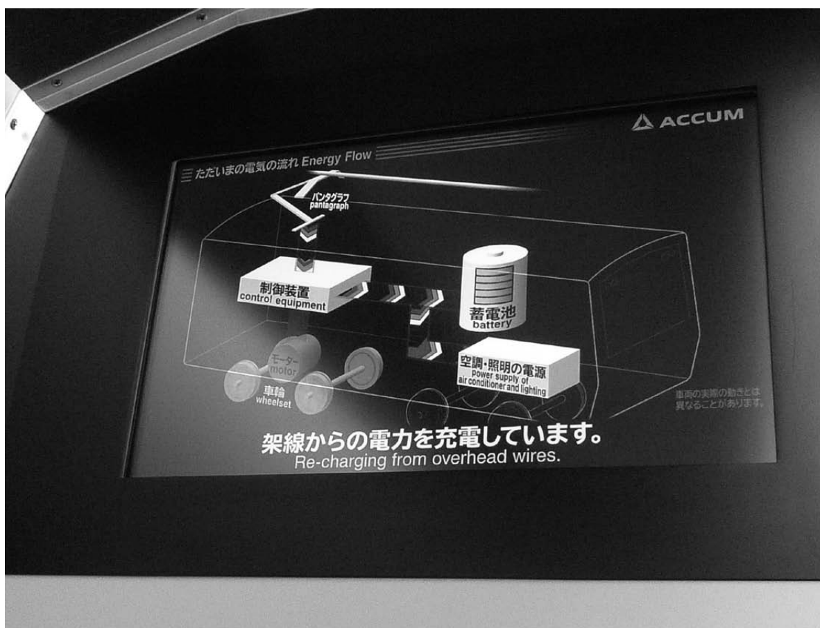
On board display showing energy flow
