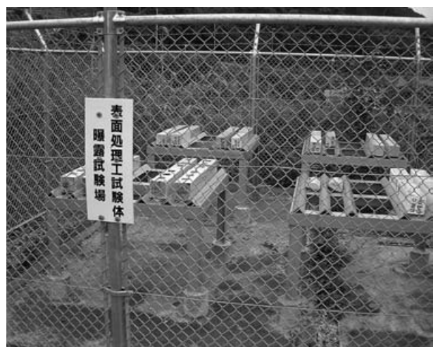
On-site weathering tests of repair materials
