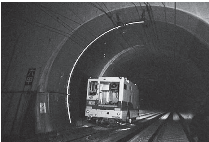
Tunnel lining surface imaging vehicle
