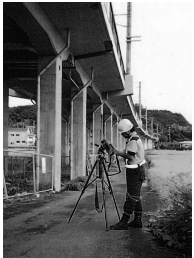
Infrared camera for detecting concrete delaminations
