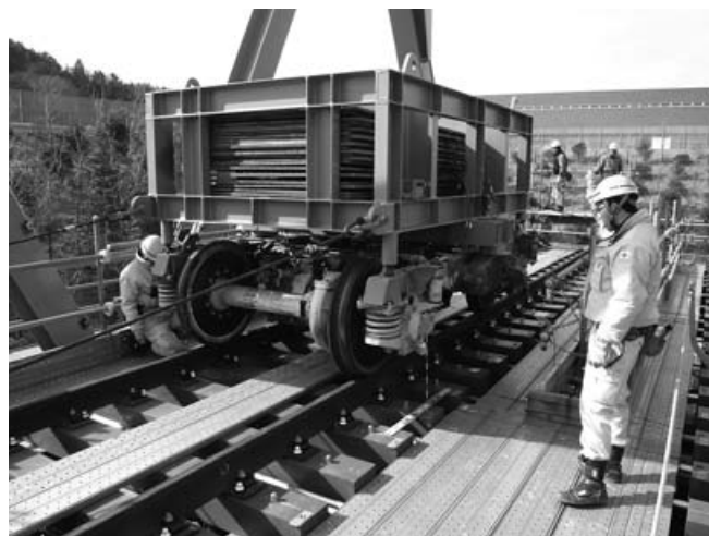
Dynamic load testing with shinkansen bogie
