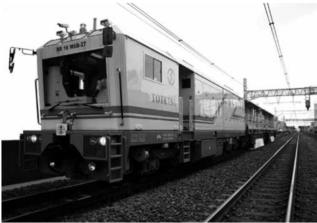
Rail grinding car
