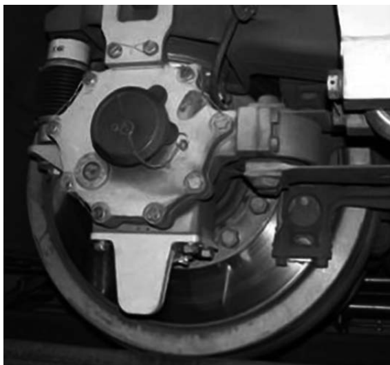
L-shaped guide (Also refer to Figure 13 on page 39) (JR East)
