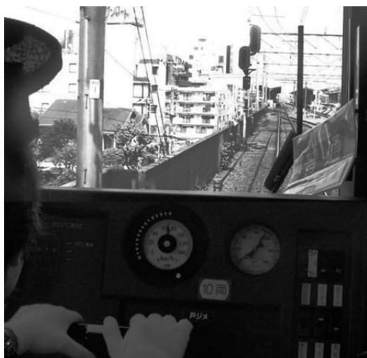
Testing is being done on digital ATC for commuter lines that allows intervals between trains to be kept to a minimum. Maximum operation speed is displayed in the cab. The signal ahead is not lit. Photo taken on May 2010, on the Keio Sagami-hara Line. (Author)
