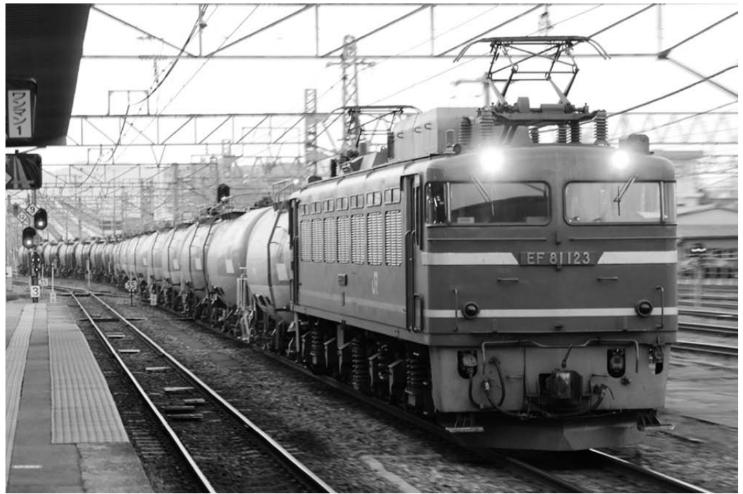
Class EF81 freight locomotive hauling tanker wagons
