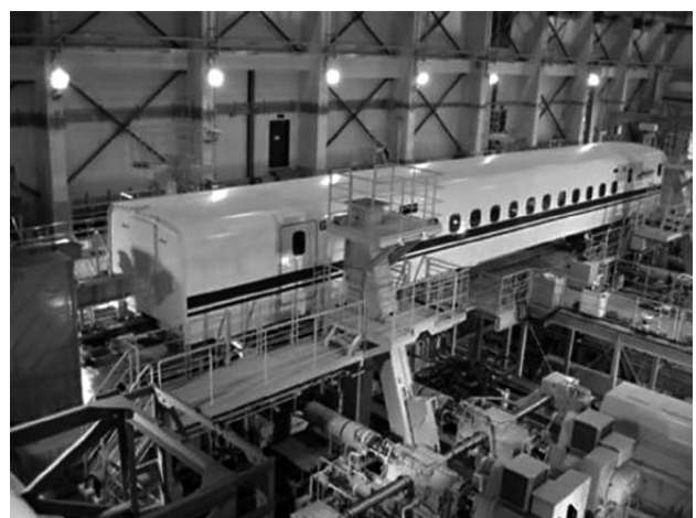
Figure 3 Vehicle Dynamic Simulator (left) and Rolling Stock Field Test Simulator (right)
