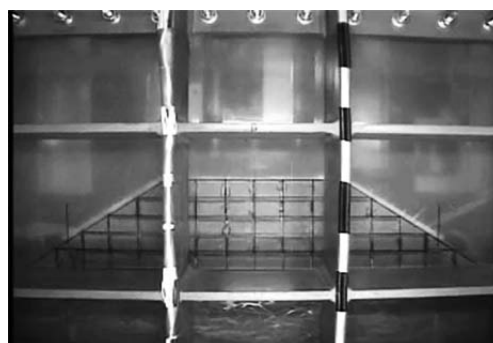
Reinforced by sheet piling (after vibration)
