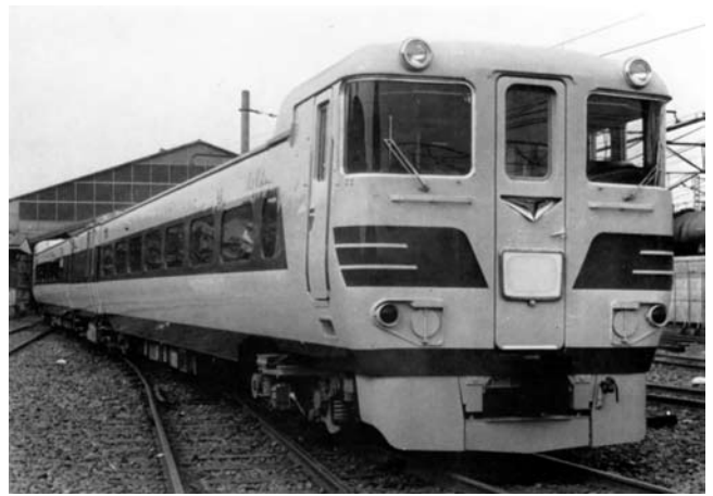
Test Series 391 Pendulum DMU (A Hundred Years of Progress in JNR Rolling Stock)
