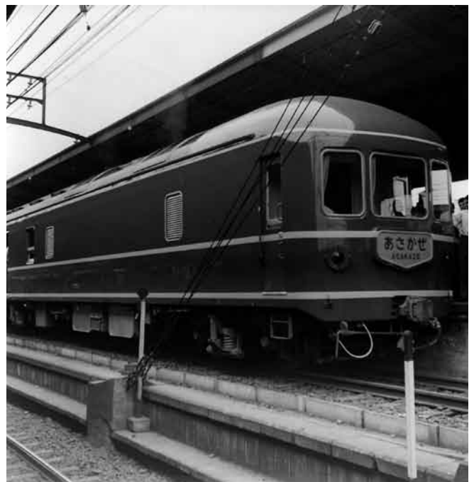
The other end car of Asakaze with power generator for lighting and air-conditioning (The Railway Museum)
