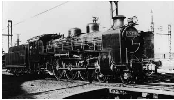
Modified version of Class C51 with smoke deflectors (The Railway Museum)
