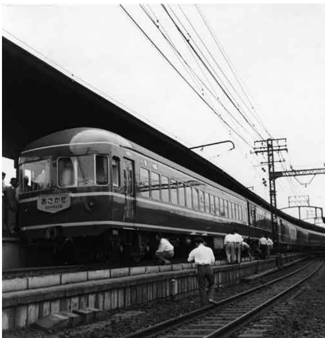
End car of Asakaze limited express (Tokyo–Hakata) composed of Series 20 air-conditioned sleeping carriage (The Railway Museum)
