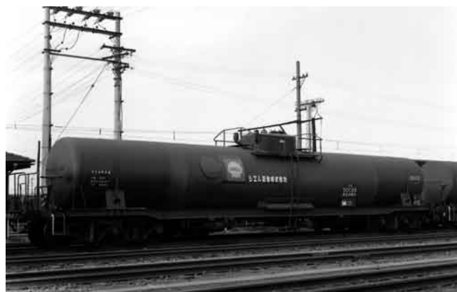
Taki 50000 tank wagon for transporting gasoline
