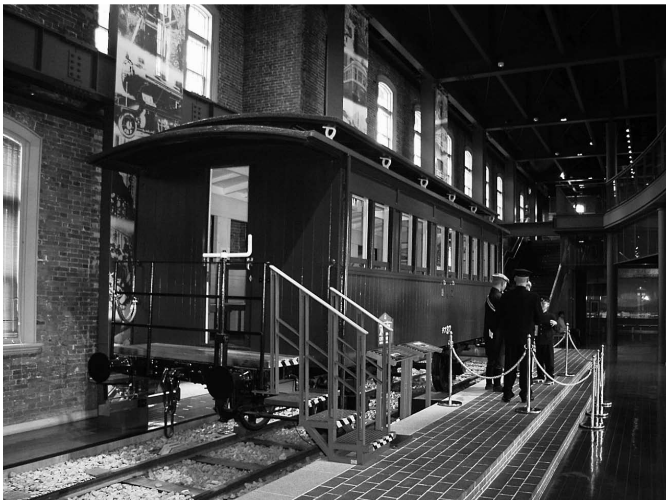
Four-wheel, third-class wooden coach built by Kyushu Railway's Kokura Works in 1897
