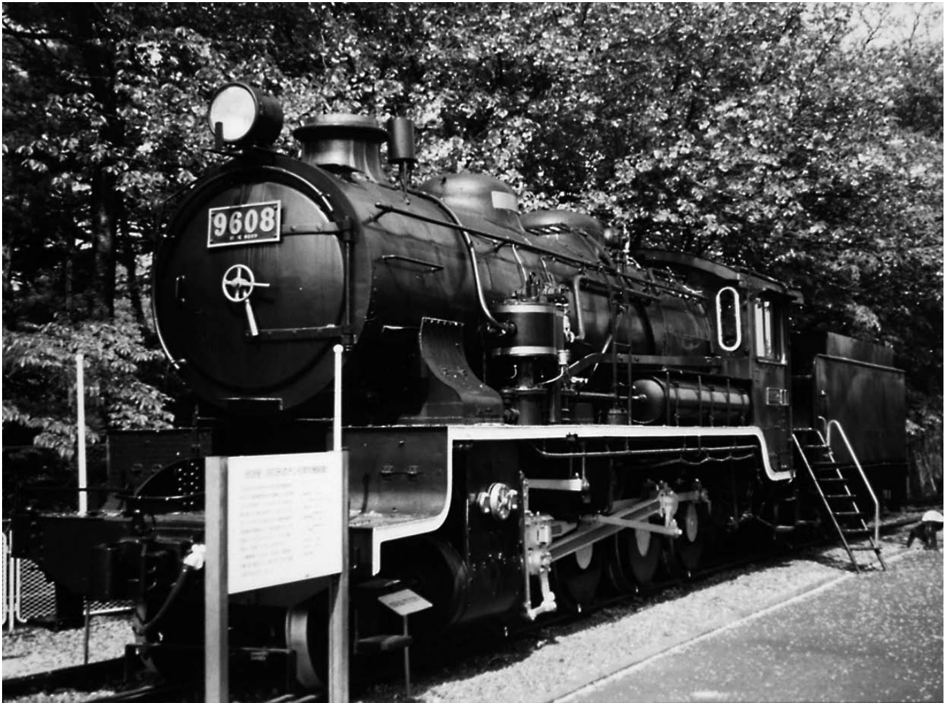
Class 9600 mass-produced tender locomotive for freight transport
