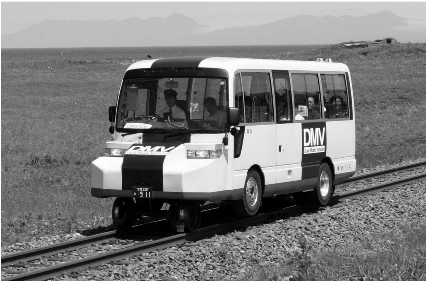
DMV911/912 running on rail
