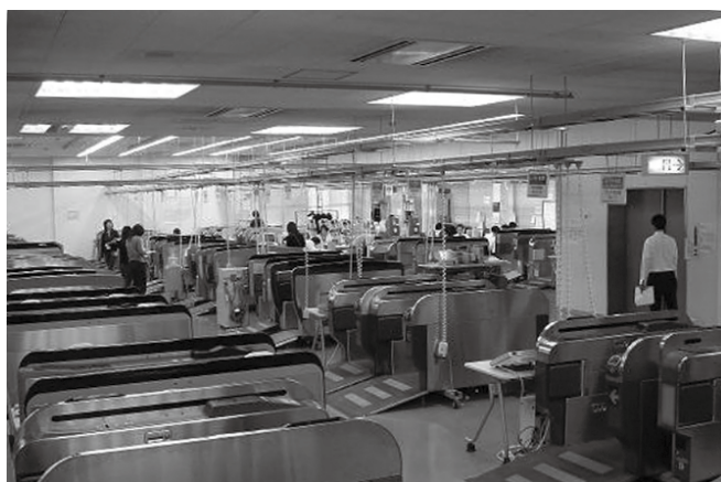
Gates (left) and ticket vending machines (right) under test at equipment test centre
