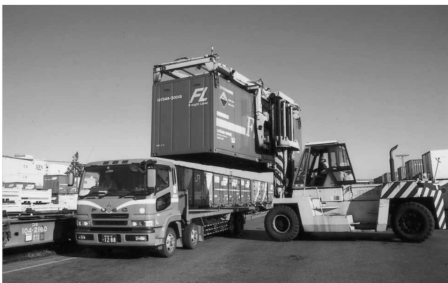
Top lifter for E&S System and larger containers
