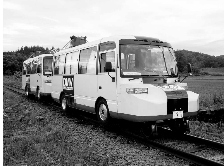
Dual-Mode Vehicle for revitalizing local lines
