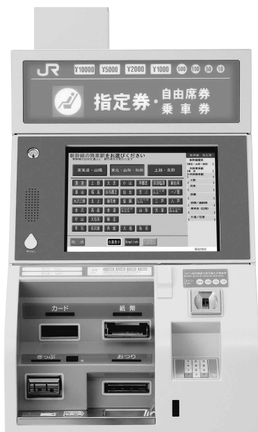
Passenger-operated MARS MV-30 terminal developed for passenger convenience and better booking-window efficiency (JR Systems)
