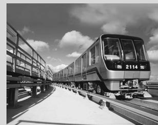
Kobe New Transit's new Series 2000 *Port Liner*. The new barrier-free stock has longer and wider body and higher ceiling to increase passenger capacity and space for luggage. (Kobe New Transit)
