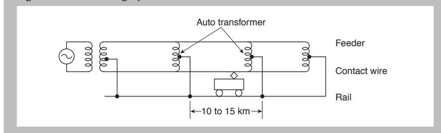
the problem was finally solved by development of the auto transformer (AT) feeding method, which does not require boosting transformers.
