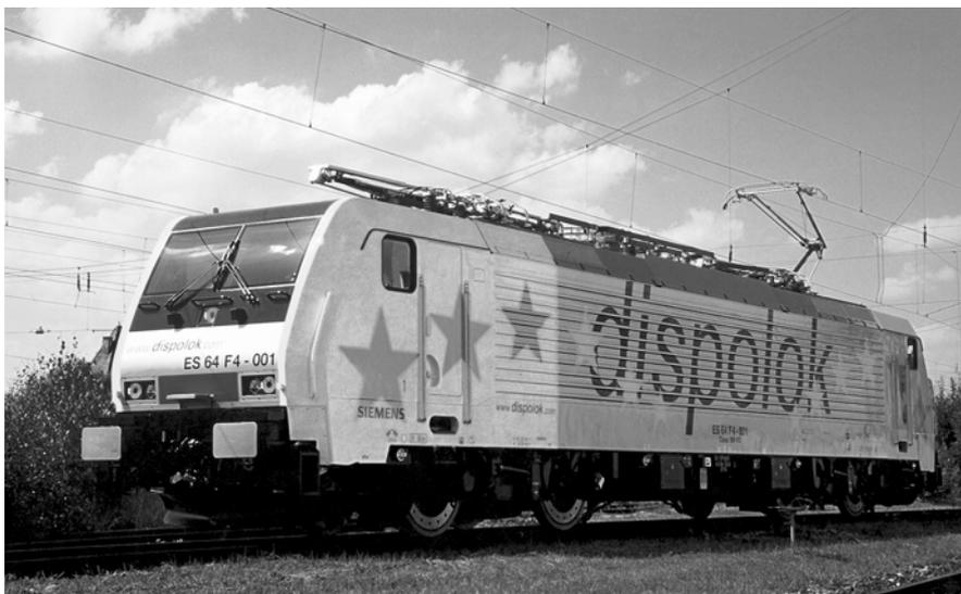
Electric four-system high-performance locomotive ES64F4 for Siemens Dispolok GmbH, Germany (STS)
