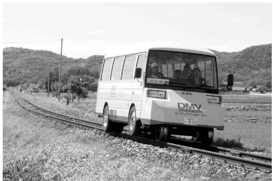
JR Hokkaido's Dual Mode Vehicle during test runs on the Sassho Line. This microbus-based vehicle was developed to revitalize business on under-used lines in Hokkaido. It has been in testing on commercial lines and public roads since 2004 and development of a two-vehicle coupled set is underway to strengthen future transport capacity. (JR Hokkaido)
