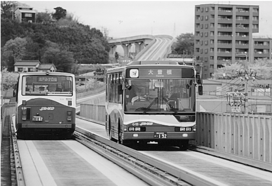
Nagoya Guideway Bus running on dedicated elevated guideway using modified buses. This new system avoids traffic congestion on normal roads to assure on-time operation. While on the elevated section, operations are regulated by the Tramway Law and a central Operations Control Room manages the bus operations as a whole. (Author)
