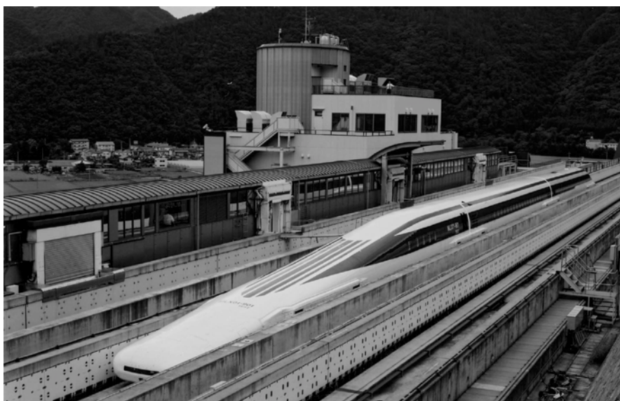
JR Central's MLX01-901 Maglev on RTRI's Yamanashi Test Track opened in 1997. The new long-nose lead carriage design was introduced in 2002 and is currently in testing. (RTRI)
