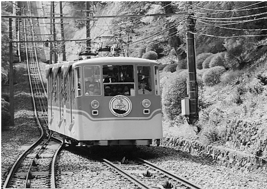
Takao Mountain Railroad's cable car operates over the highest grade (31°18') in Japan. Like many other cable cars in Japan, operations were suspended during WWII when the rails, were removed for war production, but it was restarted again in 1949. (Author)
