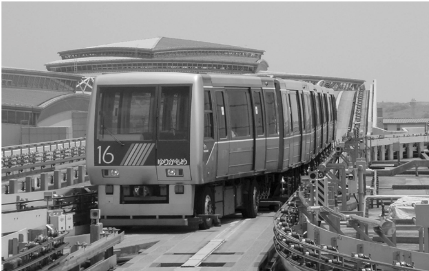
Yurikamome AGT System linking Tokyo's New Waterfront Development areas. In the 10 years since opening in 1995, it has carried 300 million people—a large number for an AGT system. A 2.8-km extension is planned to open in March 2006. (Author)
