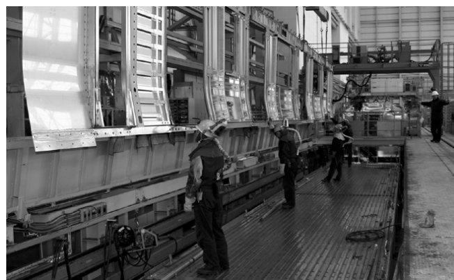
Parts are assembled into panels (for roofs, floors, etc.), which are then assembled into car bodies.
