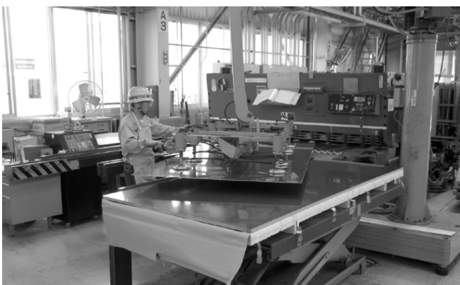
NC Machines cut and bend sheet metal for car bodies.
