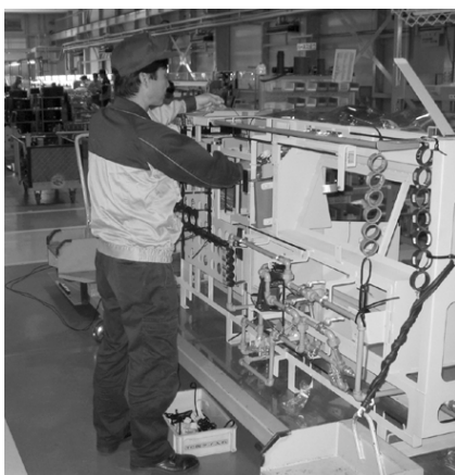
Parts such as pipes and wiring are manufactured based on NC data.
