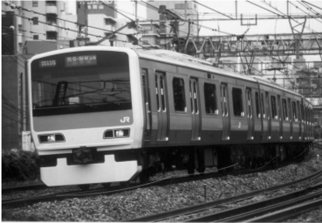
Commuter Series E231. Although the standard formation is 4M6T with four doors on each side, this train on the Yamanote Line has a 6M5T formation with two six-door cars included during rush-hour periods. (JR East)
