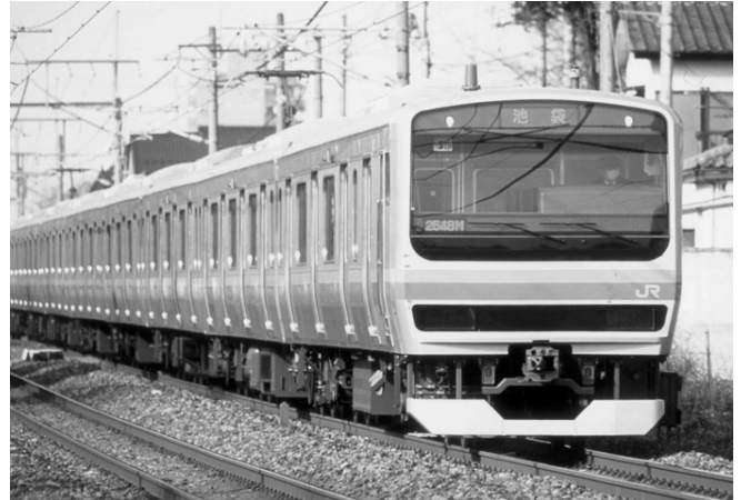
Suburban Series E231. Some seats are cross-compartment and the driver's compartment is reinforced to better withstand level-crossing accidents. (JR East)
