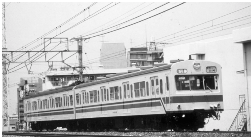
Series 101 (20-m long) introduced in 1957, combining traction system developed by private railway group and body with four 1.3-m wide doors on each side developed by JNR. This photograph shows the Series 101 on the Nambu Line, the last line on which it ran. (JR East)
