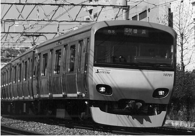
Sagami Railway's Series 10000. This is an example of minimum design changes made to the Series E231 to suit the private operator's specifications. (Sagami Railway)
