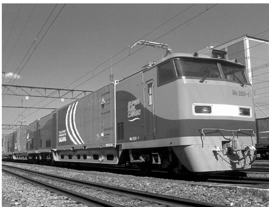
Series 250 EMU with two powered cars at each end and 12 intermediate trailing flat wagons (JR Freight)
