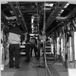
Workers at JR East Niitsu Rolling Stock Manufacturing Factory, installing in-carriage equipment such as information display, etc., in Series E231 (Photo: JR East)
