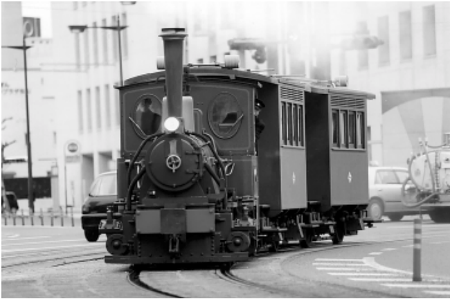
Restored special tourist train hauled by diesel engine resembling steam locomotive on suburban tracks of Iyo Railway (Author)
