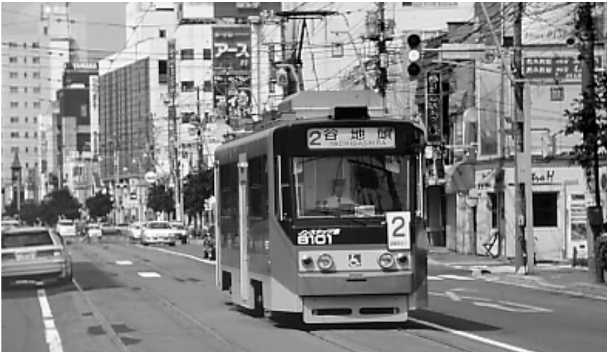
Series 8100 partial low-floor tram of Hakodate City Transportation Bureau
