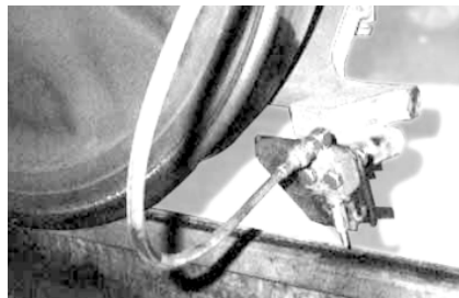
Photo 5: Bogie-mounted greasing mechanism (JR East)
