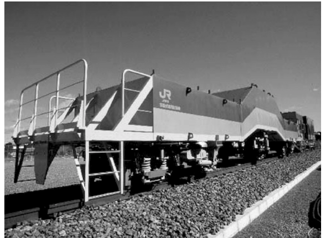
Track and Structural Dynamics Simulator—full-scale track test under real shinkansen bogie (JR Central)
