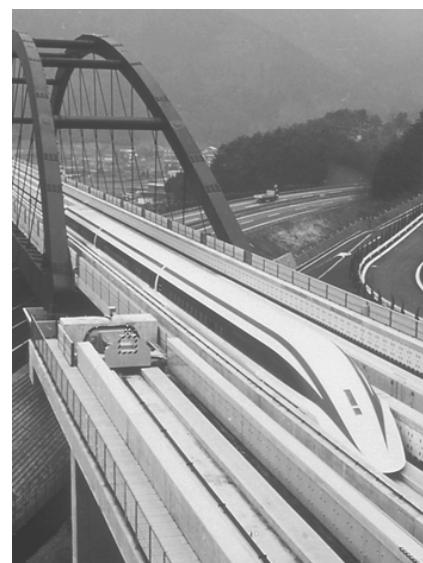
Superconductive magnetically levitated linear motor car running on Yamanashi Test Line (RTRI)
