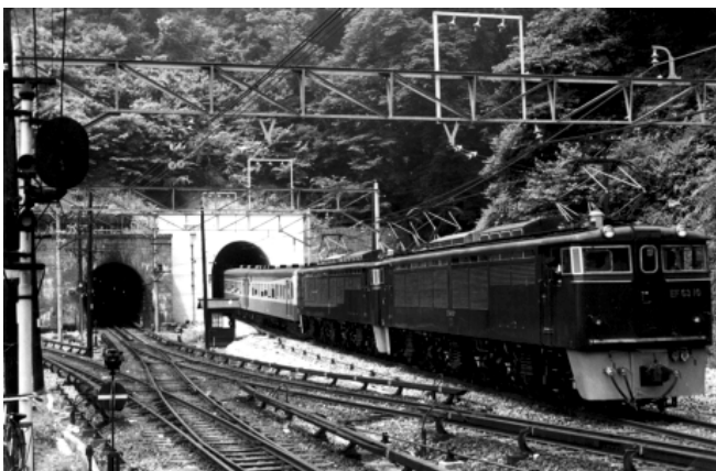
The Usui Pass was always a hurdle for rail transport on the Shin'etsu main line. In later days, JNR coupled two Series EF63 electric locomotives at the back to push trains up the grade until the section was abandoned in 1997. (Transportation Museum)
