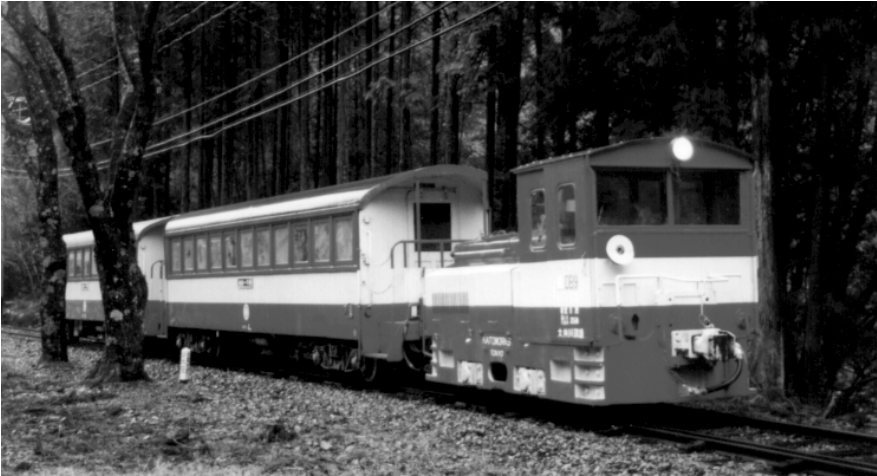
Oigawa Railway's Class DB1 locomotive and carriages on Igawa Line. The 25.5-km line on the northern section of the Oigawa Railway contains many curves with journey time of 1 h 45 minutes. Its rolling stock is smaller than traditional ones with width of 1.8 m. (S. Takashima)
