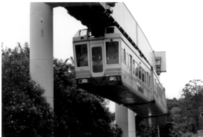
The suspended Shonan Monorail (Safage) was constructed as a technology demonstration by Mitsubishi. (Y. Kato)
