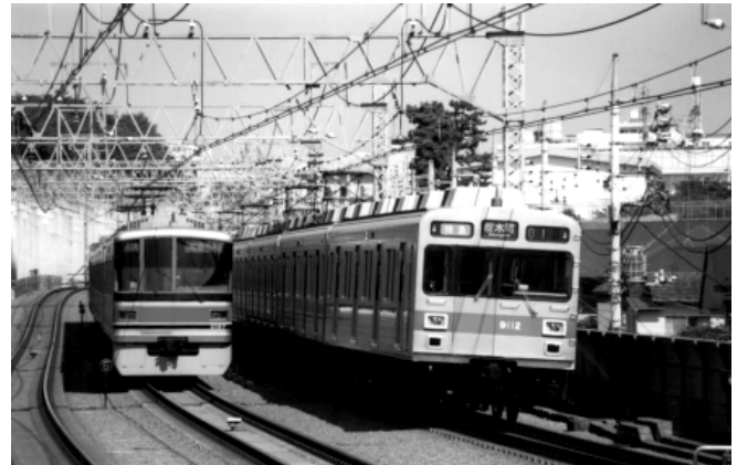
Tokyu's limited express train on Toyoko Line (right) and local train on Meguro Line (left) running parallel on quadruple-track section. The Meguro Line started operation to reduce congestion by improving the infrastructure. (S. Tominaga)
