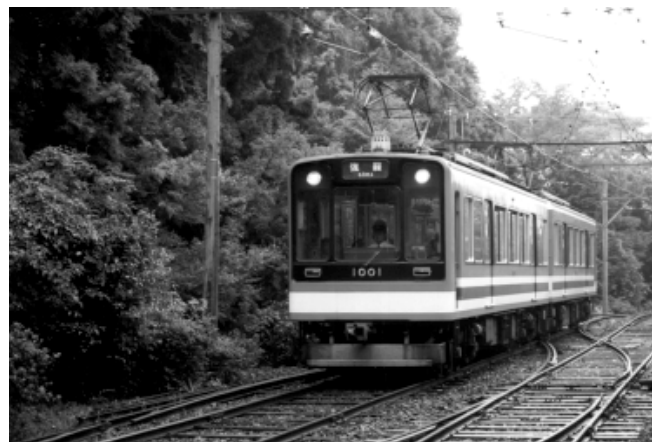
Hakone Tozan Railway's Series Kumoha 1000 running through one of Japan's most popular tourist spots. There are many sections with 80 per mill, which is the highest grade that can be handled without using a rack-and-pinion system. (Y. Kato)
