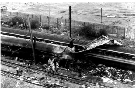
Ladbroke Grove: The dark patch of ground in front of the DMU shows where wreckage of the destroyed leading car burned after its fuel tank burst. This was the highest collision speed ever recorded for a head-on collision. (B. Morrison)
