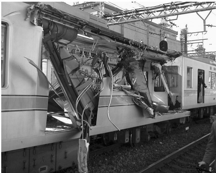
TRTA's Hibiya Line train derailed and was hit by on-coming train, killing five people (8 March 2000). (MLIT)
