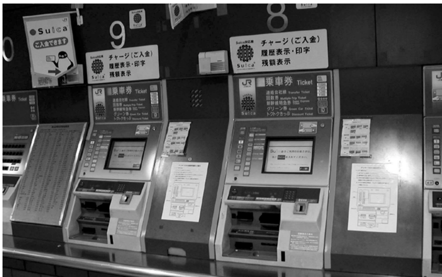
These machines can check and print the Suica SF amount and usage history as well sell magnetic tickets. (JR East)
