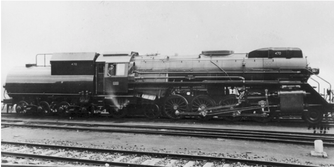
The NSB Class 49 four-cylinder compound was a true super-power locomotive. This example (No. 470) is preserved in static condition at the Norwegian Railway Museum. (Krupp, Norwegian Railway Museum Collection)
