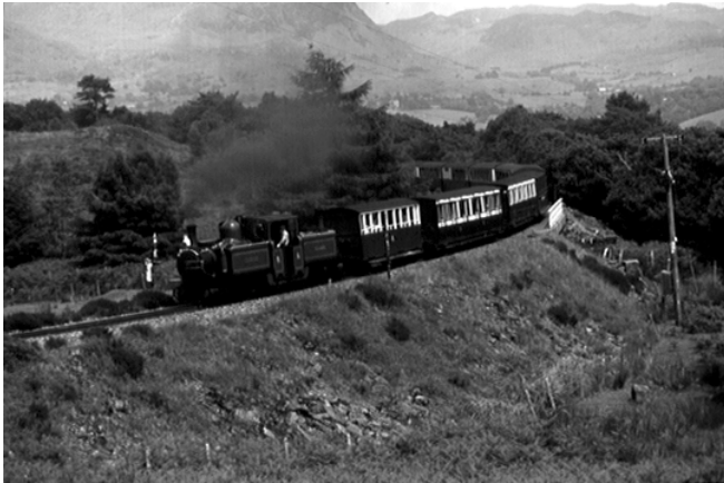
Fairlie replica loco chugging gallantly up the continuous grade of 10 to 15 per mill at more than 40 km/h on the loop line at Duart just like the original 130 years ago. (Author)
