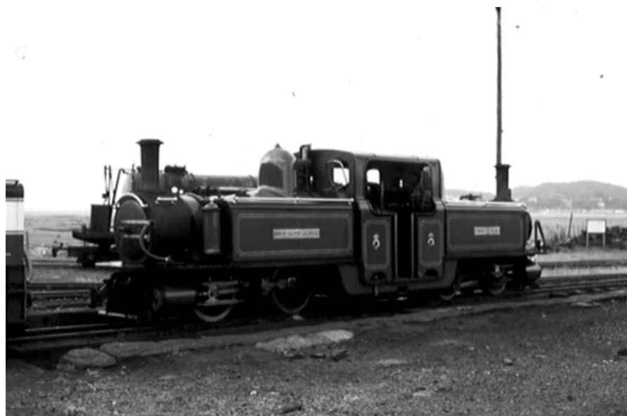
Working replica of Fairlie's Little Wonder double-boiler locomotive. The only difference from the original is the cab roof—the original did not have one. (Author)
