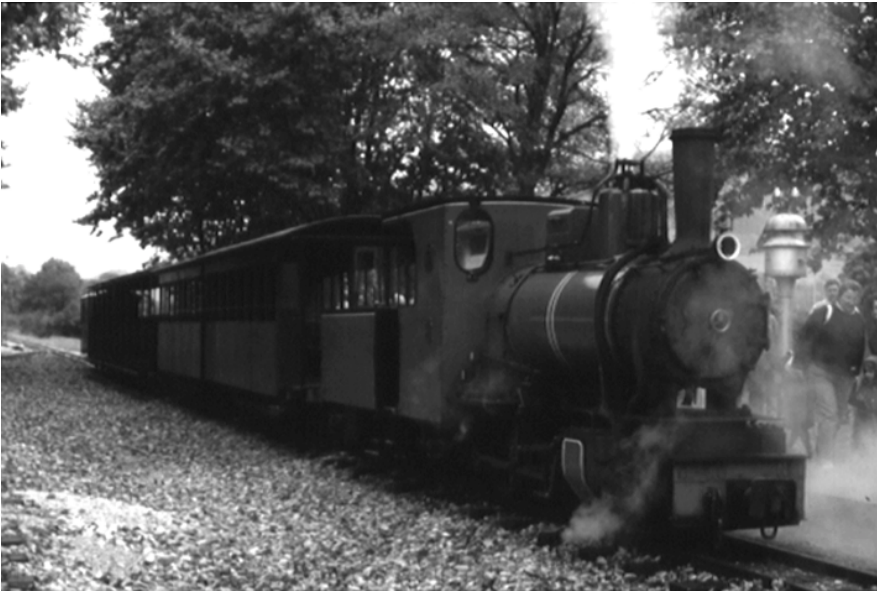
Decauville 020 (0-4-0) steam engine with home-made tender on narrow-gauge ARVO Railway in Burgundy rebuilt on abandoned standard gauge railway (Author)
