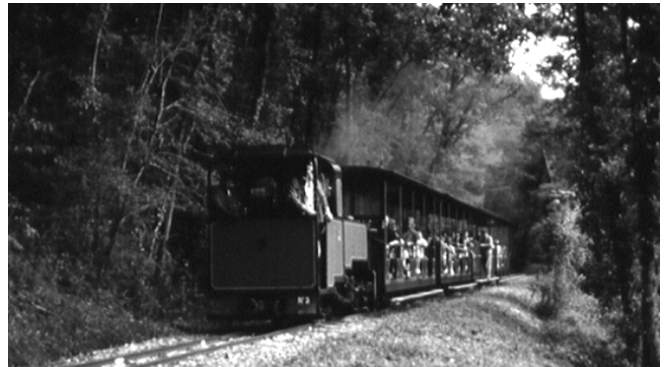
Unusual 50-cm gauge Tarn Tourist Railway with Decauville 030 T (0-6-0 T) rebuilt on site of abandoned local 60-cm gauge railway (Chemin de fer touristique du Tarn)
