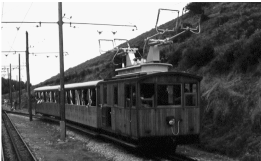
Splendid wooden electric loco on La Rhune meter-gauge rack-and-pinion track near Biarritz (Author)
