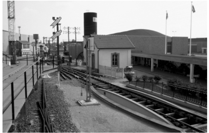
The French National Railway Museum in Mulhouse presents all the elements of a railway line, including signal box, signals, water tower, water crane, weighbridge, buffer stops, turnouts, guards hut, bridge, etc., in a small open-air space. (Author)
