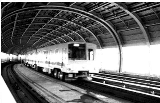
Sapporo City's Namboku Line Series 3000 EMU with rubber tyres running inside the snow shelter (Sapporo City Transport Bureau)
