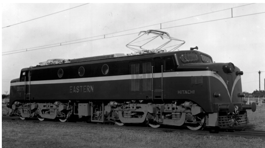
One of the first three Japanese DC locomotives (3000 V, 3600 hp) exported to the Indian Railway in 1958 (Hitachi, Ltd.)
