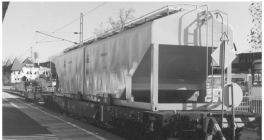
Basket car loaded with 88-m 3 self-discharging modules for bulk materials
