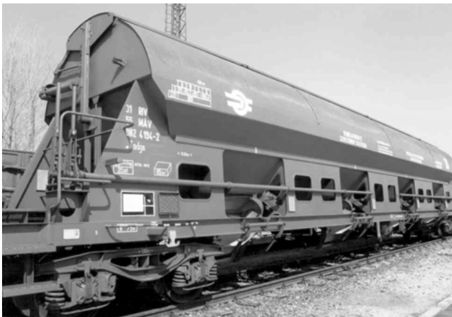
80-m 3 self-discharging wagon for bulk materials (cereals)
