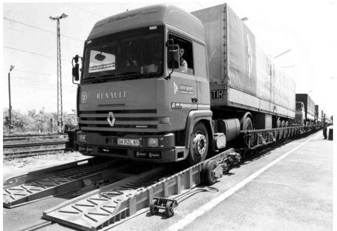
Intermodal Ro-La wagon for piggyback transport
